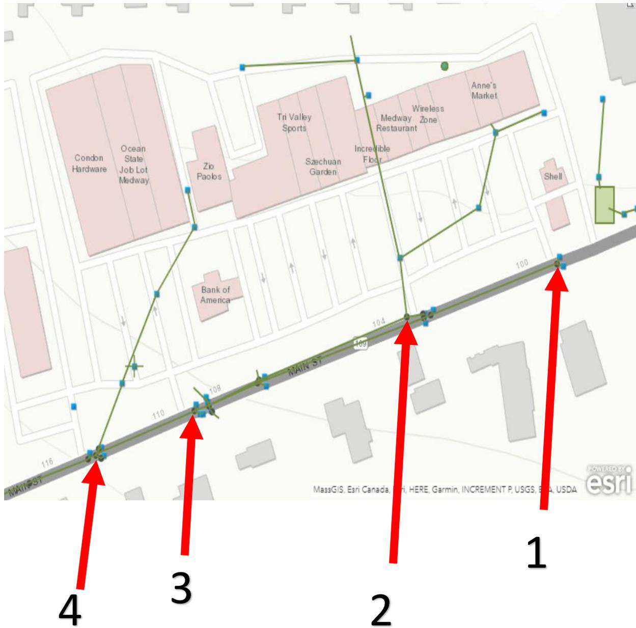
Location 1: Topographical peak. Test this location to determine stormwater composition before it interacts from Medway Plaza's discharge.
