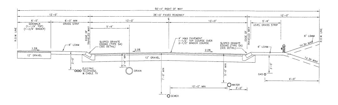
NOTE: WHEN HYDRANTS ARE PROPOSED ON THE SIDEWALK SIDE OF THE ROADWAY THE HYDRANT MUST BE LOCATED ALONG THE BACK OF WALK, WITHIN ROADWAY LAYOUT IN ACCORDANCE WITH CURRENT ADA/AAB STANDARDS.
