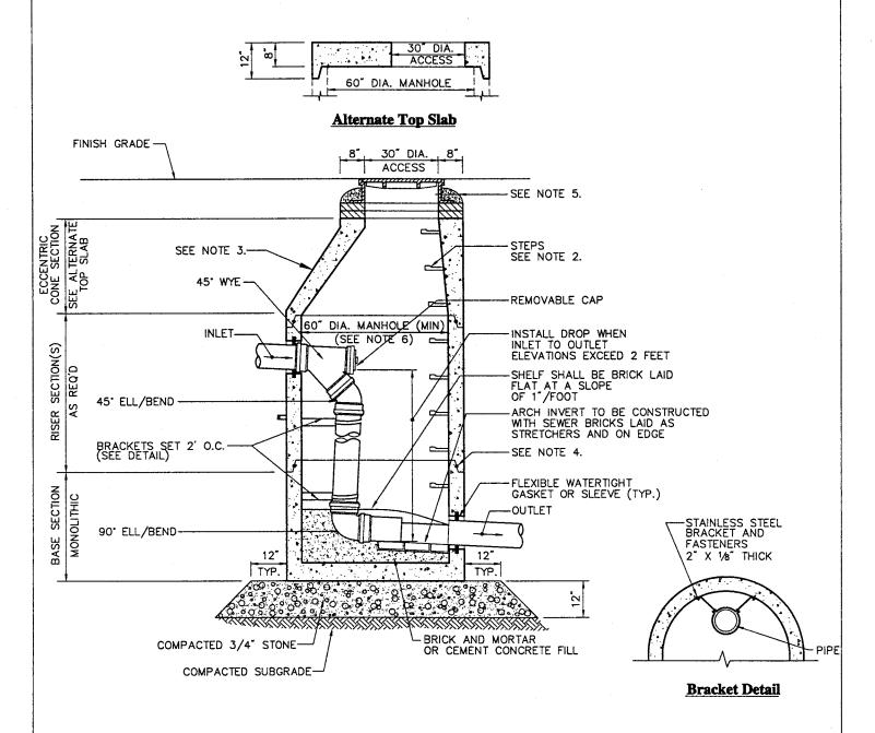
INTERIOR DROP SEWER MANHOLE DETAIL
