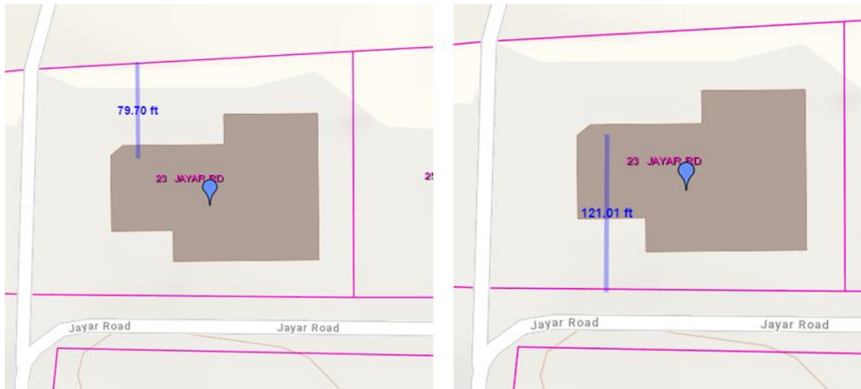
Figure 2. Distance of proposed rooftop HVAC unit to property lines
