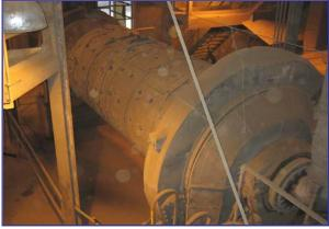
Ball Mill Wrap with exposed liner bolts at a cement plant.
