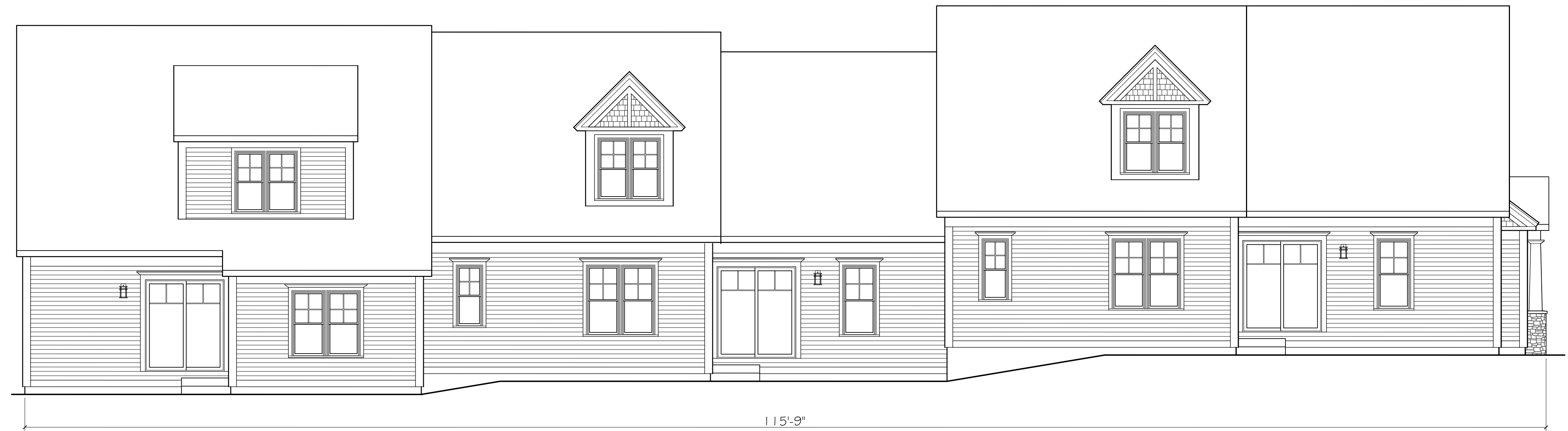
Preliminary Left Side Elevation - Units 3, 2 and 1 Scale: 3/16" = 1'-0"
