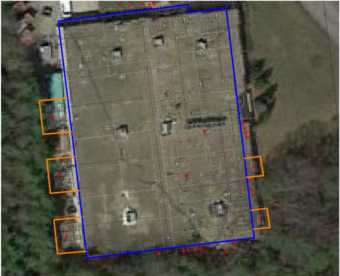
FIGURE 3. Recommended Noise Control Solutions, Barriers shown in Orange around GRTUs and AHUs
