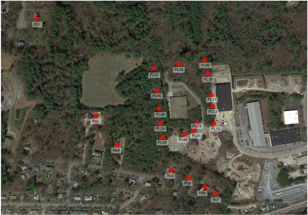
FIGURE 2. Computer model receptor points on source property line and beyond
