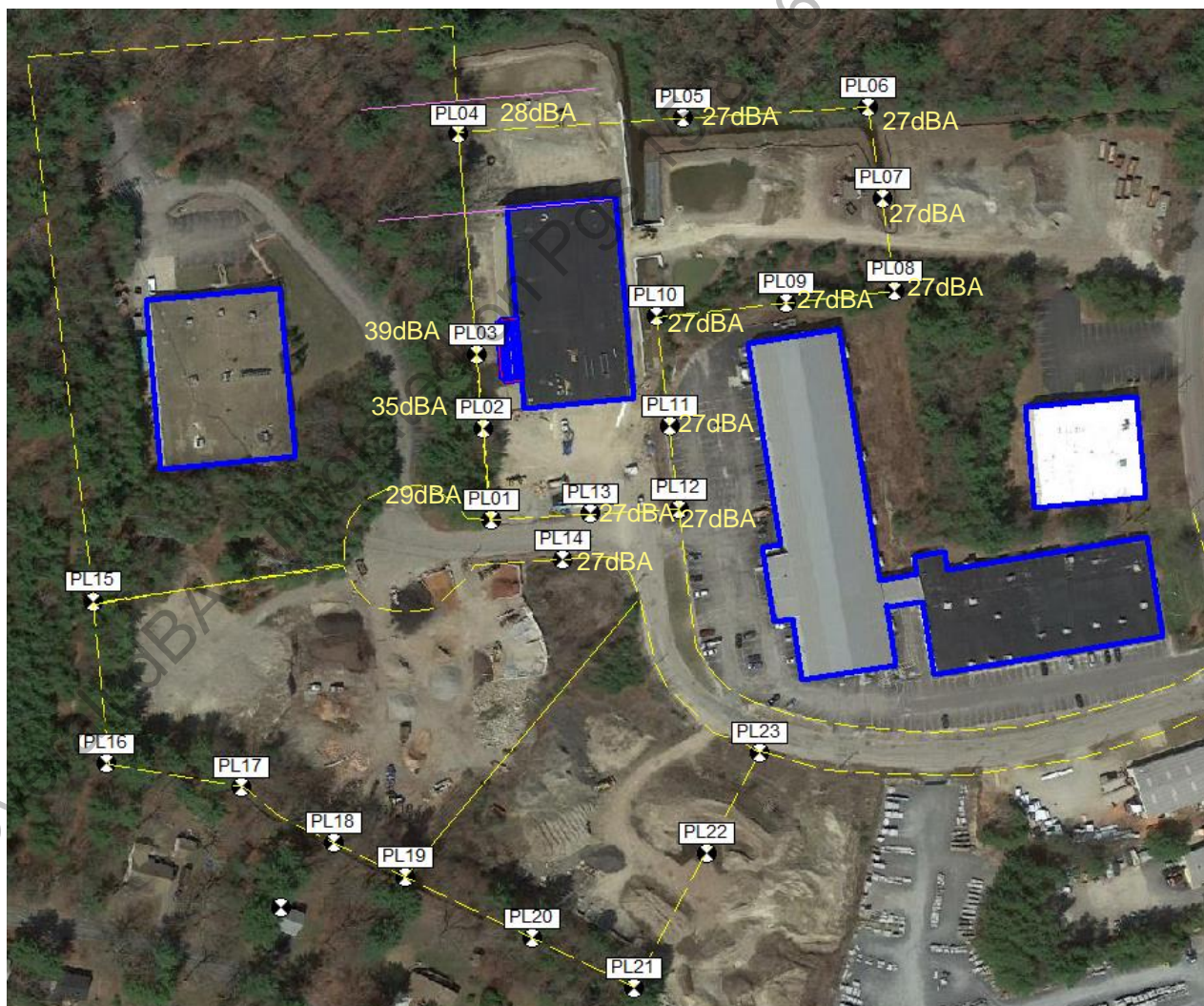
FIGURE 2. Receptor points on source property line (see TABLE II)
