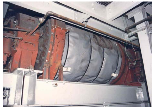
Ball mill HUSH COVER™ using HC-500S-1" with banding attachment.
