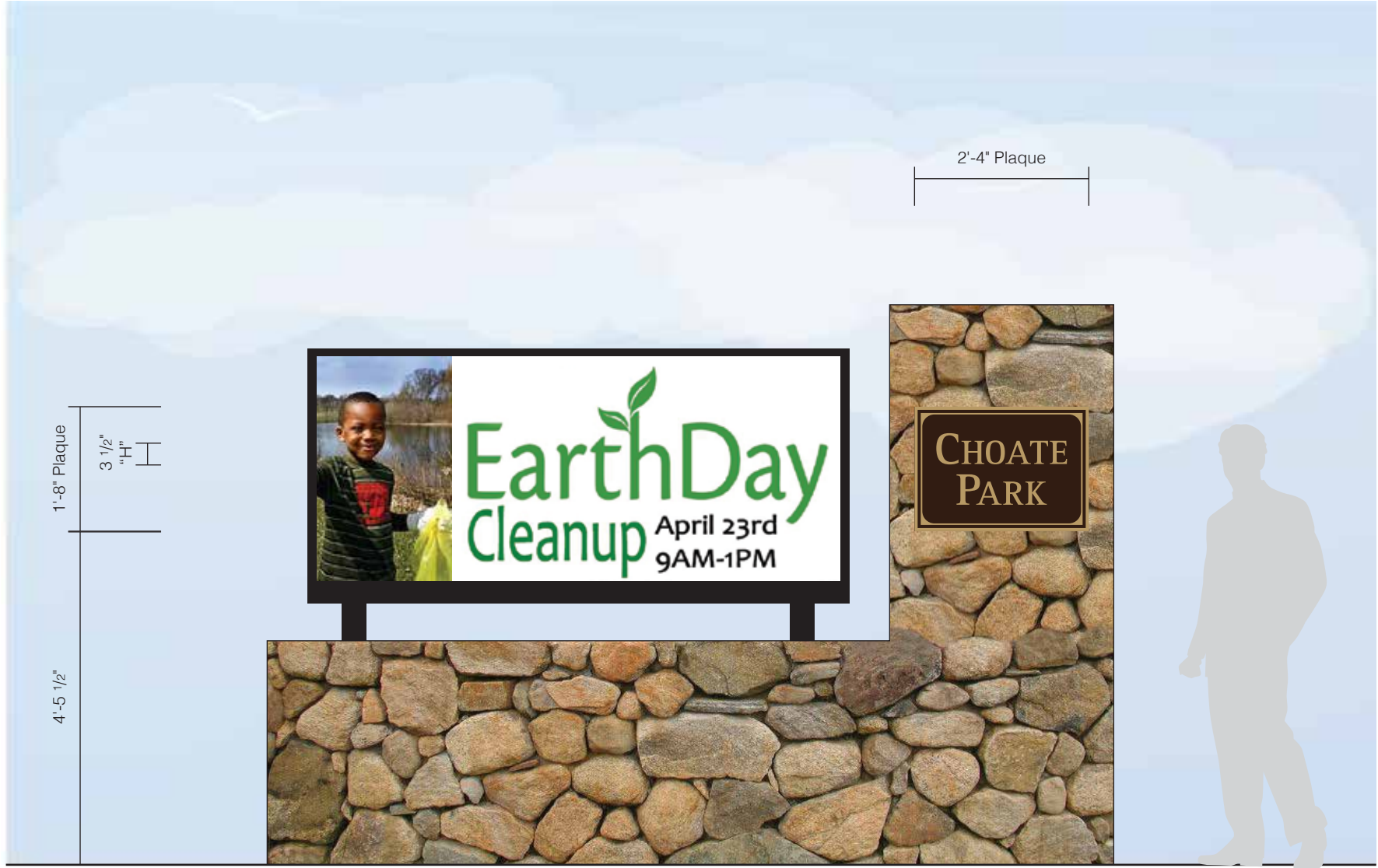
A Sign Elevation - Front View Scale: 1/2"=1'-0"
