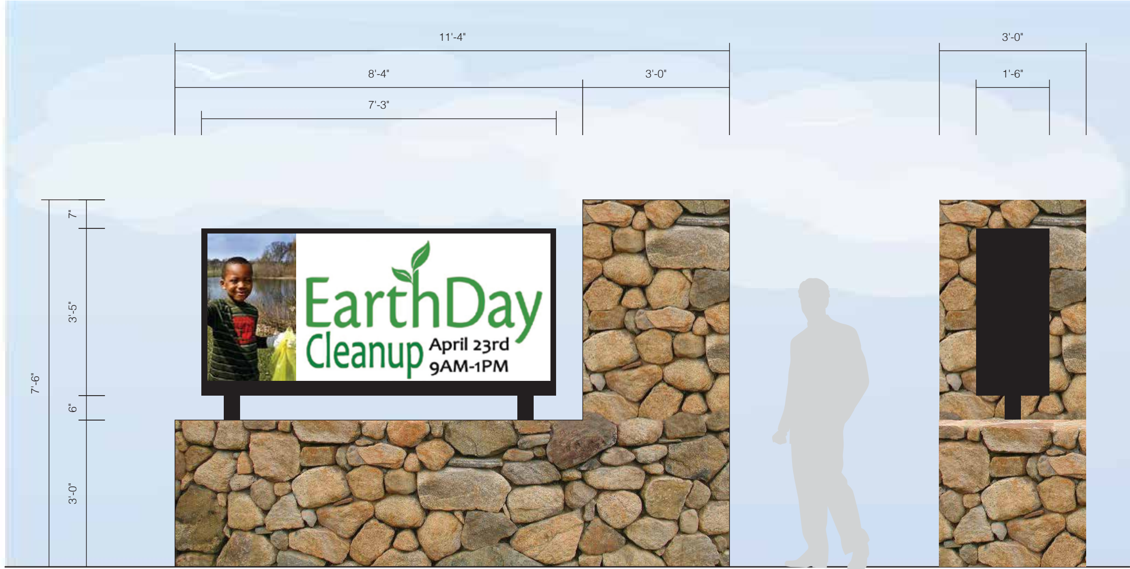
A Sign Elevation - Front View Scale: 1/2"=1'-0"
