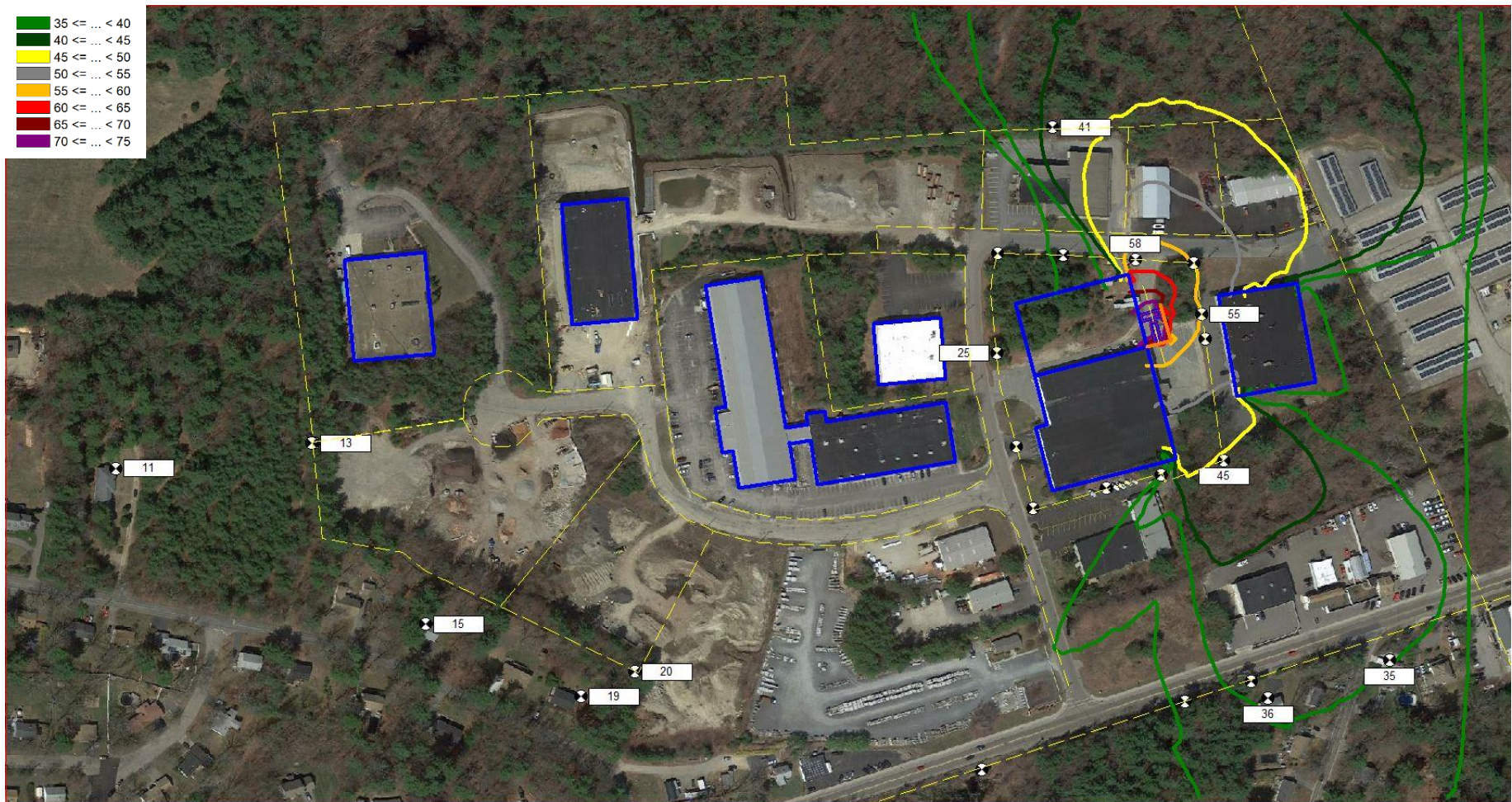
FIGURE 3. Estimated Phase 2 community sound levels, noise controls for 65 dBA facility property line limit
