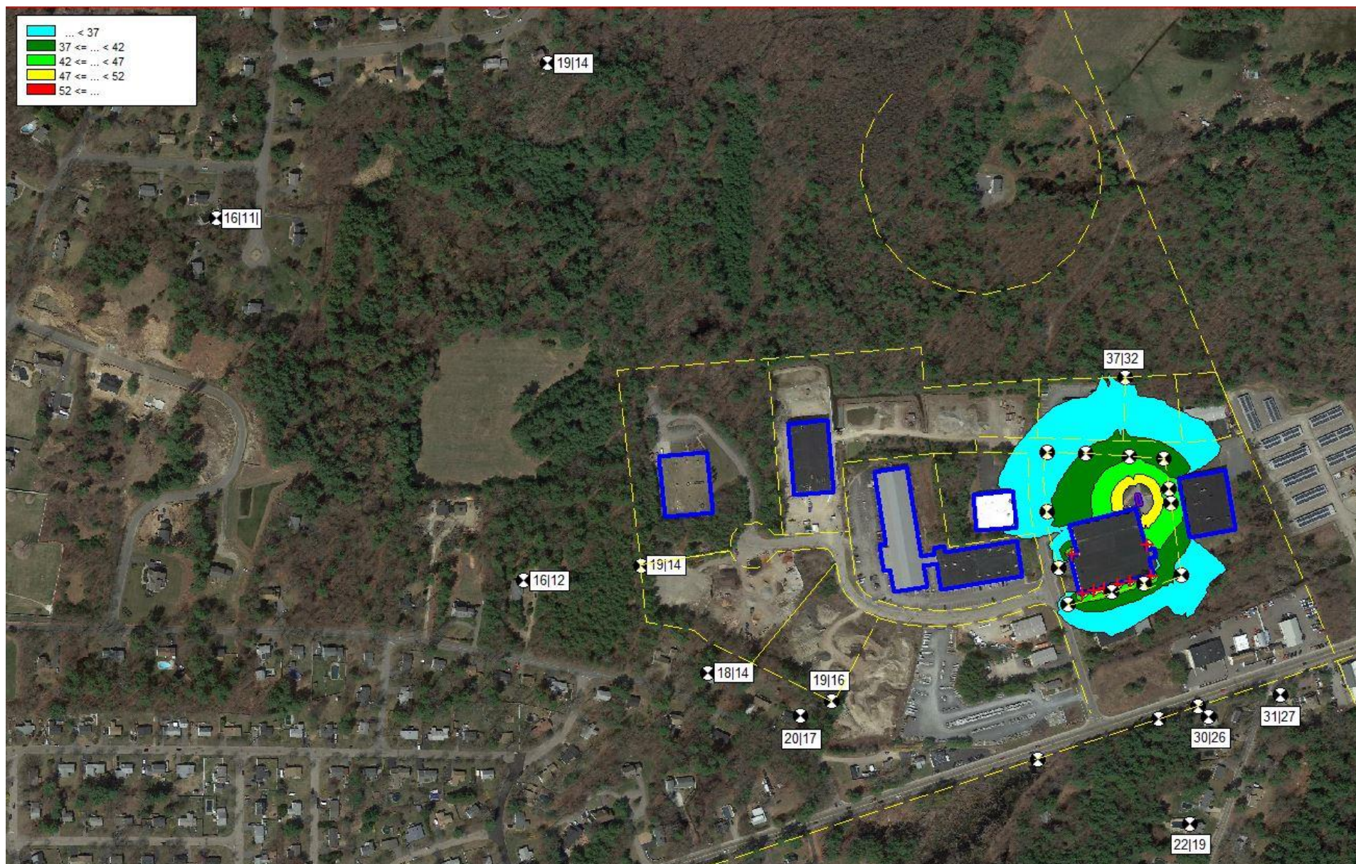
FIGURE 4. Estimated Phase 1 mechanical equipment community sound levels, night sound level contours shown in color
