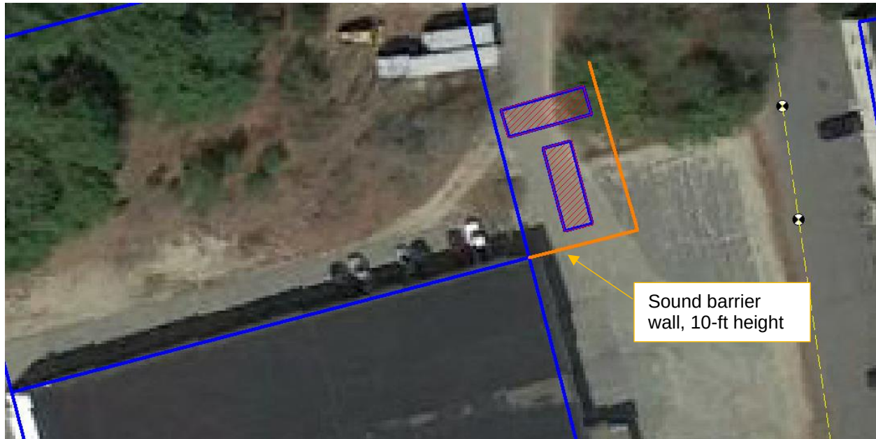
INSET 1. Barrier configuration for 65 and 60 dBA facility property line design goals
