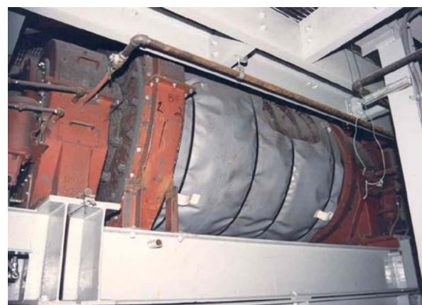
Ball mill HUSH COVER™ using HC-500S-1" with banding attachment.
