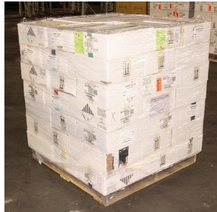
Figure 2-4: Li-ion polymer pouch battery pallet layout; top view shown on left and elevation view shown on right.
