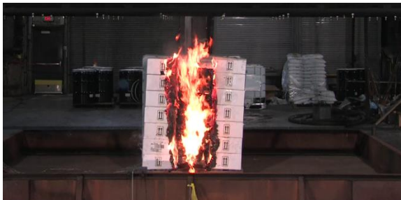
46 min 0 s – secondary ignition
