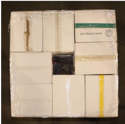
Figure 2-4: Li-ion polymer pouch battery pallet layout; top view shown on left and elevation view shown on right.
