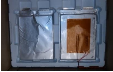
Figure 5-4: Photos of heater placement within ignition carton. Left photo shows a foil heater affixed to a battery on the fifth level (of ten levels) within the carton. Right photo shows the heater wiring exiting the carton.
