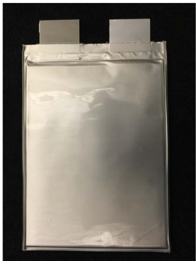
Figure 2-2: Li-ion polymer pouch battery; outside foil pouch shown on left, internal components shown on right. (images courtesy of Exponent, Inc.)
