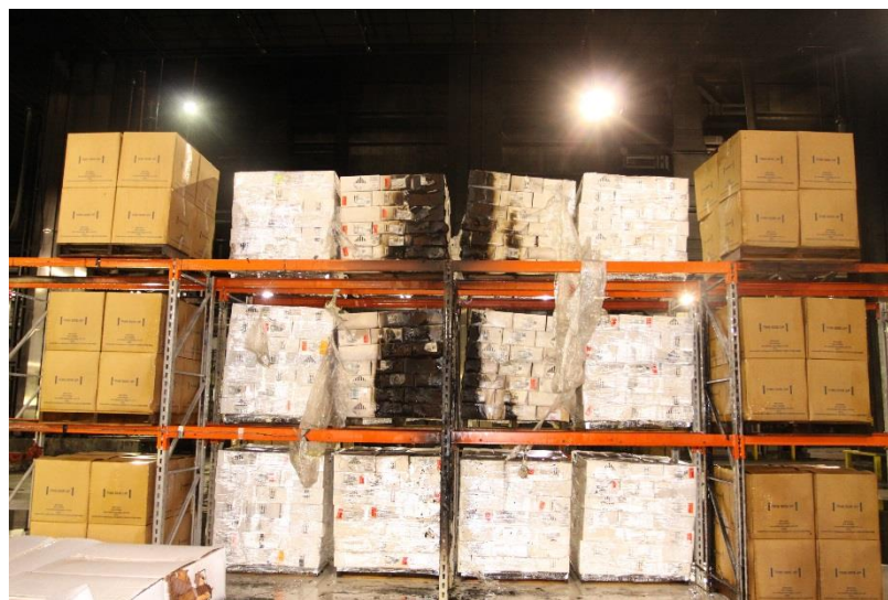
Commodity across longitudinal flue
