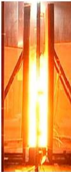
Figure 6-1: Photo demonstrating the fire spread in a parallel panel configuration (left) and plot of overall heat released as a function of the water flow rate for various ignition sizes (right). Courtesy of Thumuluru and Xin.
