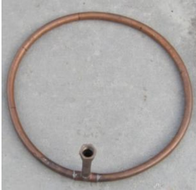
Figure 3-2: Propane ring burner (left) within the rack and fire size within rack (right).
