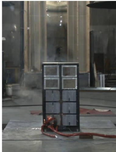
Figure 4. Intermediate-scale free burn test set up. Courtesy of FM Global.
