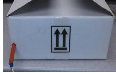
Figure 5-4: Photos of heater placement within ignition carton. Left photo shows a foil heater affixed to a battery on the fifth level (of ten levels) within the carton. Right photo shows the heater wiring exiting the carton.
