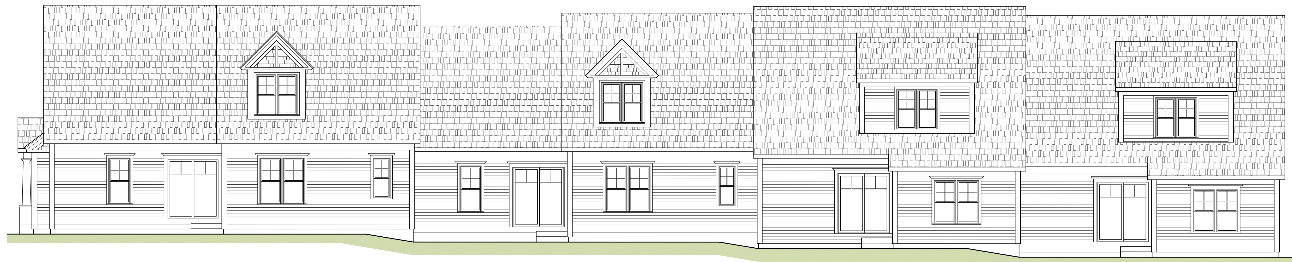
Preliminary Rear Elevation - Units 4, 5, 6 and 7 Scale: 3/16" = 1'-0"
