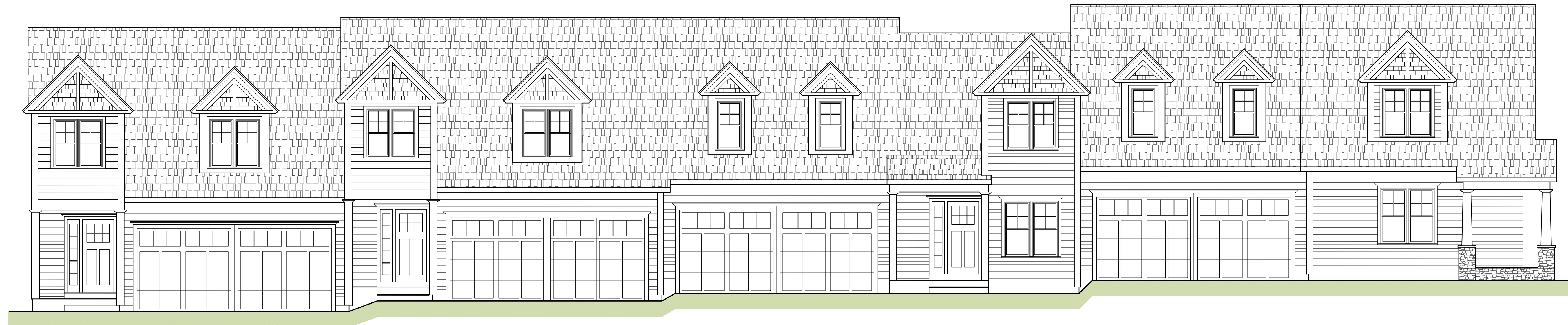
Preliminary Front Elevation - Units 4, 5, 6 and 7 Scale: 3/16" = 1'-0"
